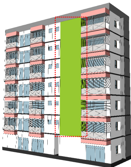
Figure 19: Image 02_ Case Building selected for simulation assumed with green façade on south wall of the building
